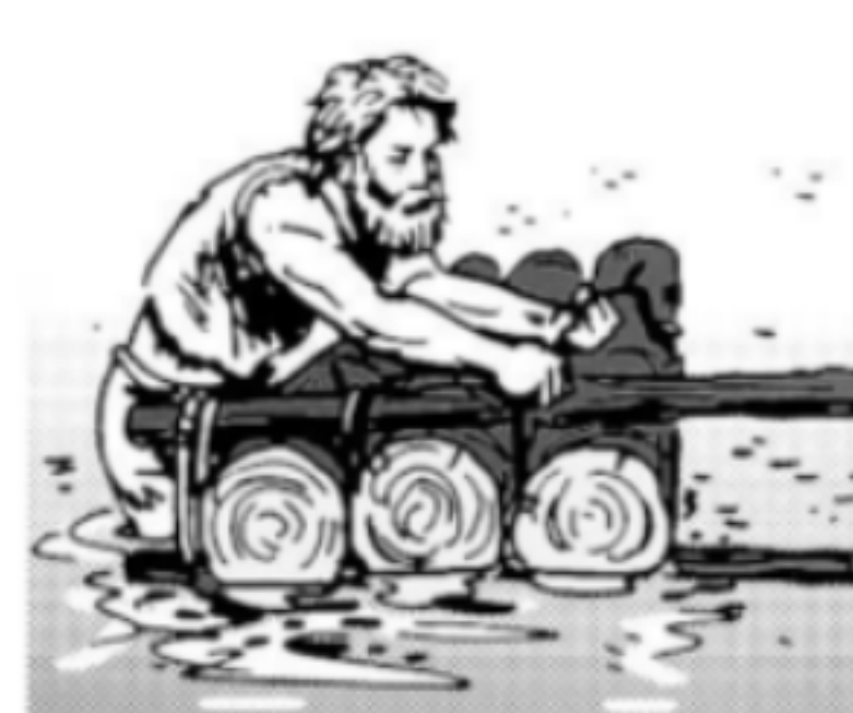
3: SANDWICH the larger logs with 2 thin logs and use rope or thick vines to tie them in place.
