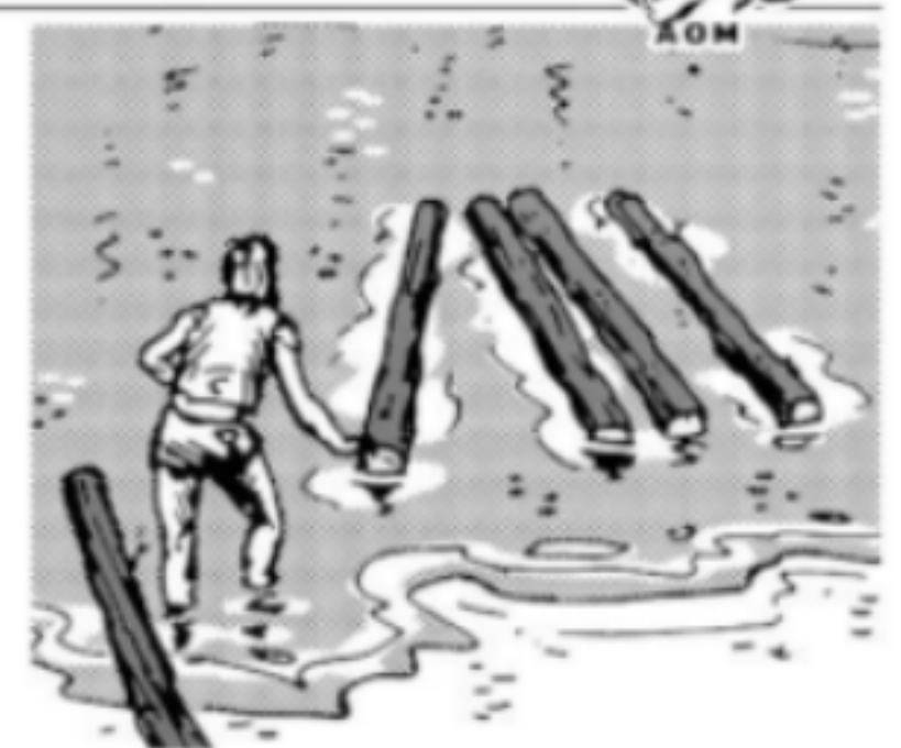
2: DRAG THE LOGS into shallow water and arrange the thicker ones next to each other to make a platform.
