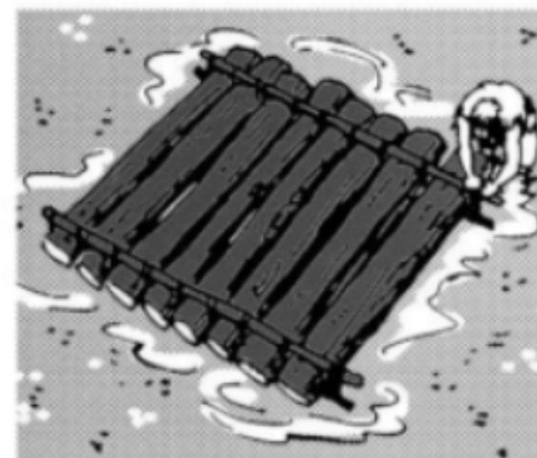
5: REPEAT ON THE OTHER SIDE, using your remaining two thin logs to secure the other side of the raft.
