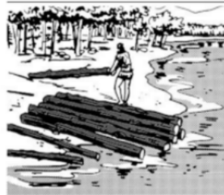
1: GATHER 6-8 10-FOOT LOGS at least 10 inches in diameter, and 4 thinner 10-foot logs at least 6 inches in diameter.
