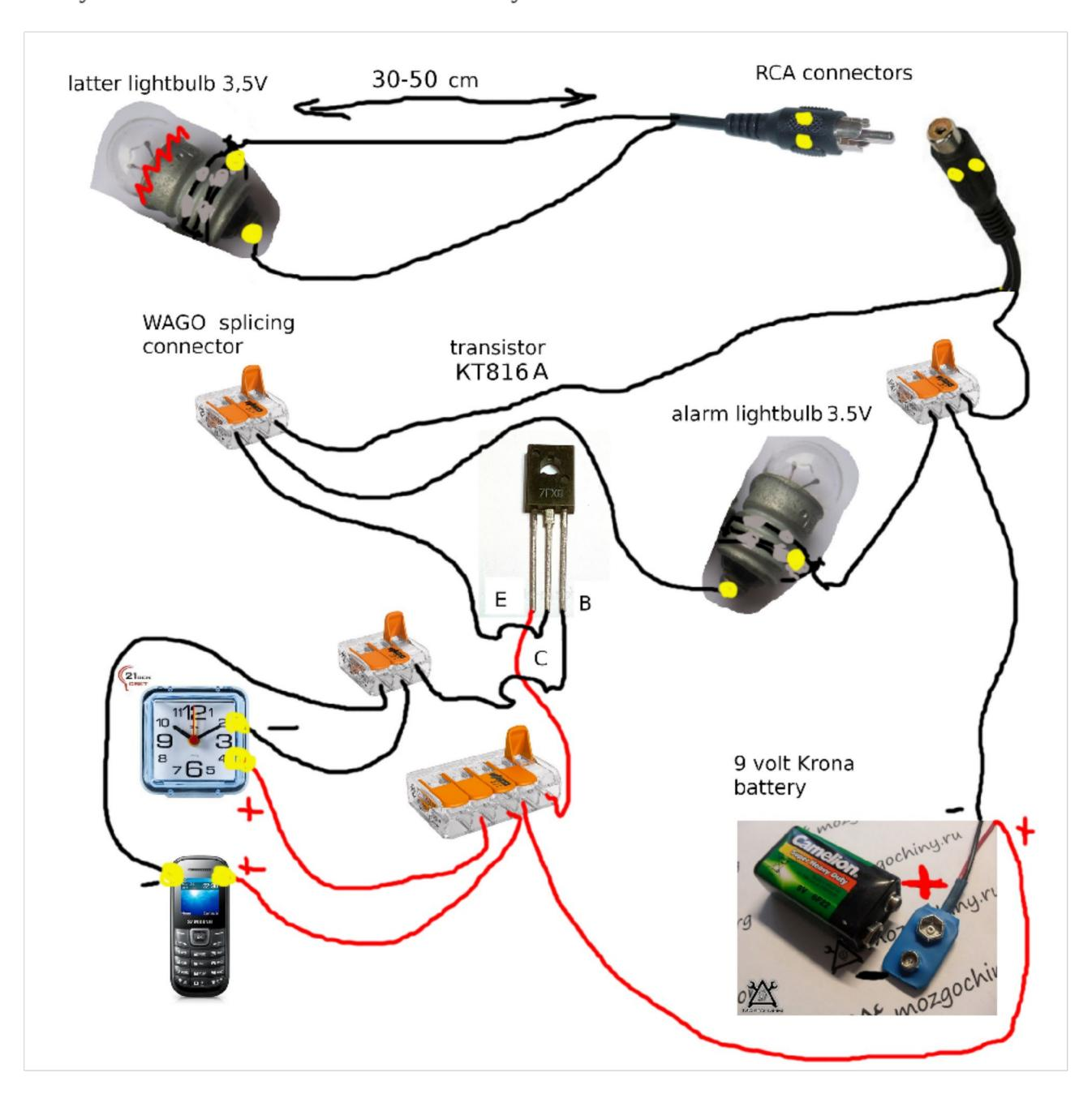
The scheme basically speaks for itself. A mobile phone/alarm clock sends a signal that opens the transistor. As a result the current starts flowing through a «prime» circuit – from a 9 volt Krona battery to the ignition device. A 3.5 volt lightbulb serves as the latter.
